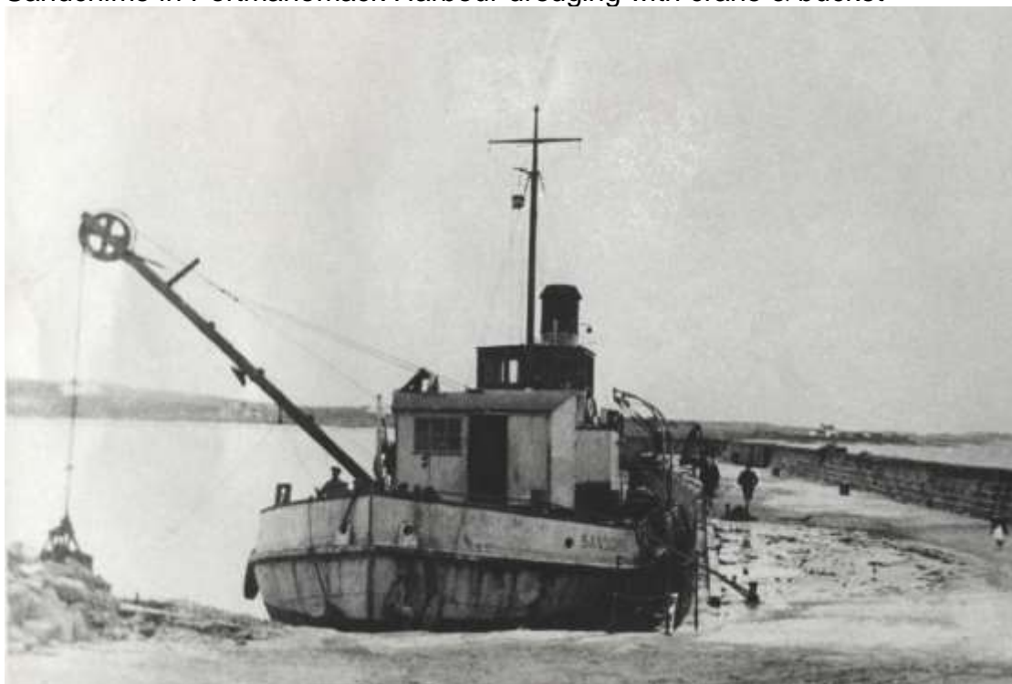
Sandchime in Portmahomack Harbour dredging with crane & bucket
