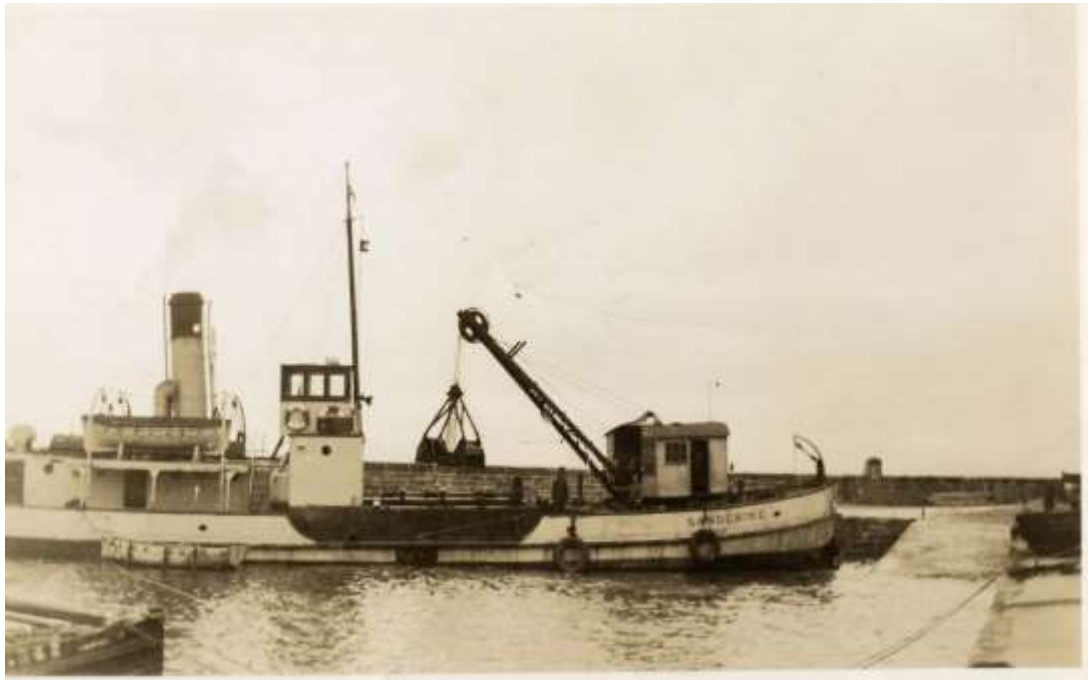
Sandchime in Portmahomack Harbour dredging with crane & bucket
